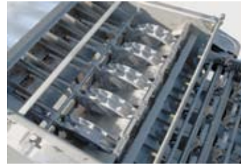
Singulating worm & feed wheel
